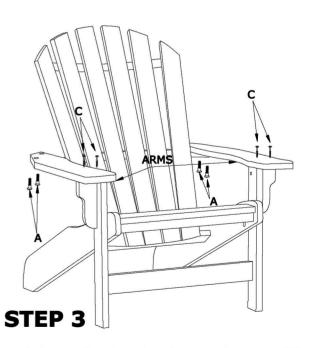
Attach Arms to front Legs from the top using screws (C). Bolt Arm Assemblies to Back Assembly using Bolts (A) as shown.
