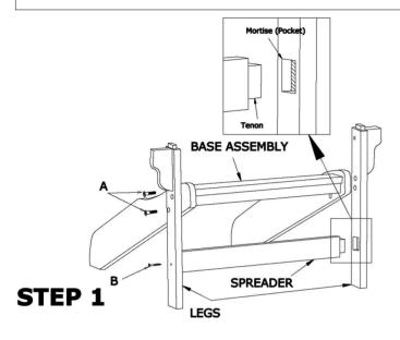
Attach Spreader tenon into mortise (pocket) on Leg Assemblies and attach with screws (B) as shown. Bolt legs to Base Assembly using bolts (A).
