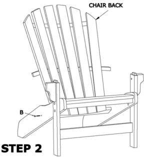
Tenons on the Back Assembly will fit into mortise (pocket) in Base Assembly. Attach with Screws (B) as shown).
